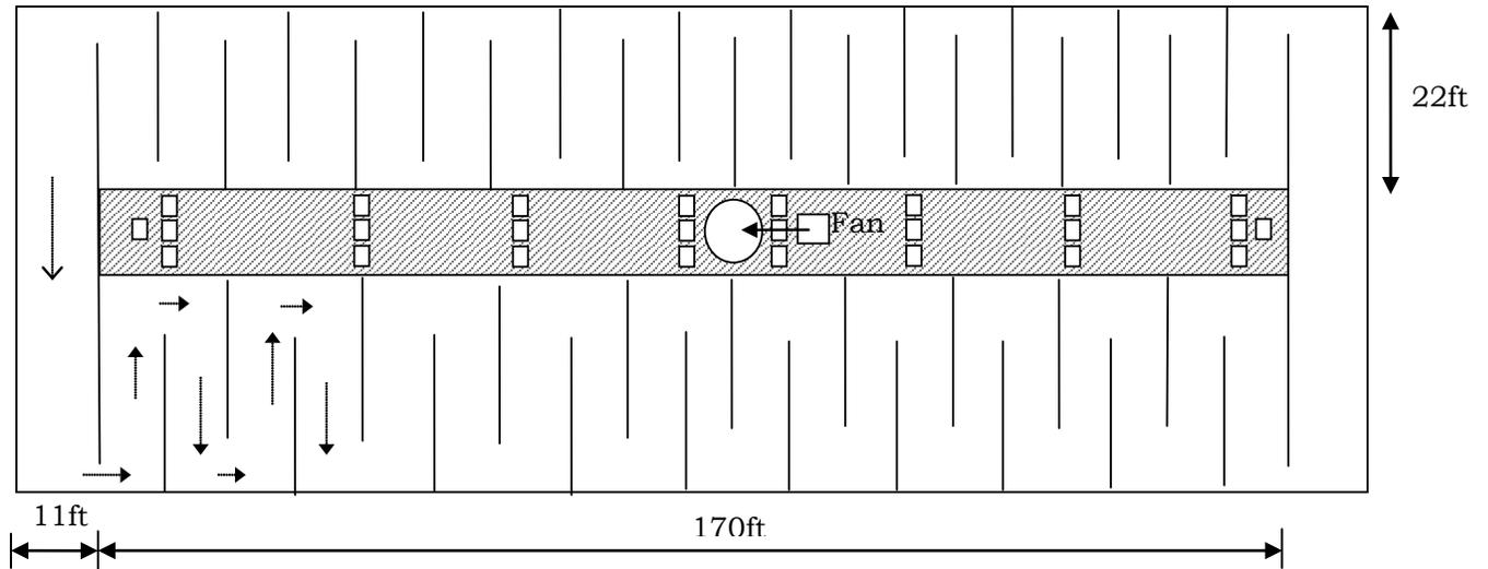
**Figure 3.3: Modified design of the monitored high draught zigzag kiln**
