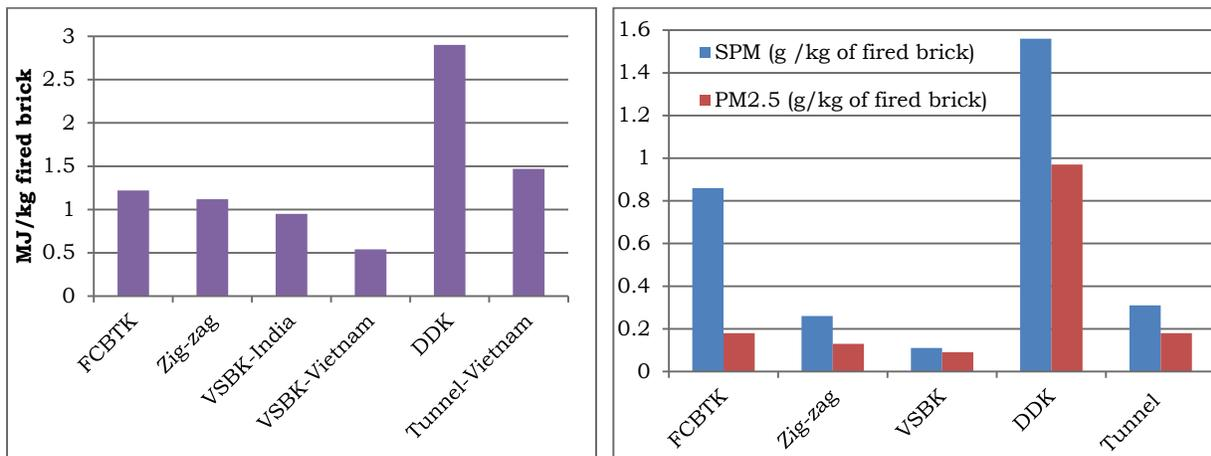
**Figure 1.1: Comparison chart of energy and emissions of five brick kiln technologies monitored in 2011**
