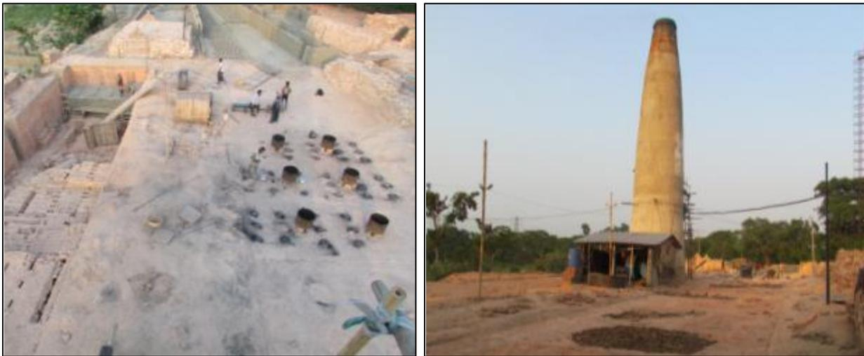
**Figure 3.4 -Monitored Modified High Draught Zigzag kilns, Howrah**
