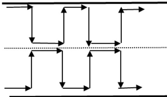
*Air flow in Zigzag kiln*
