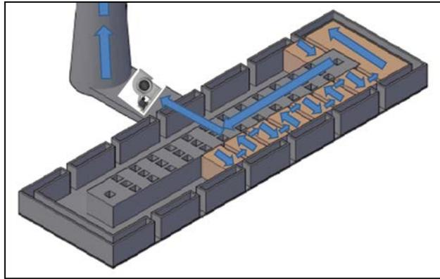
*Zigzag air flow in Zigzag kiln*
