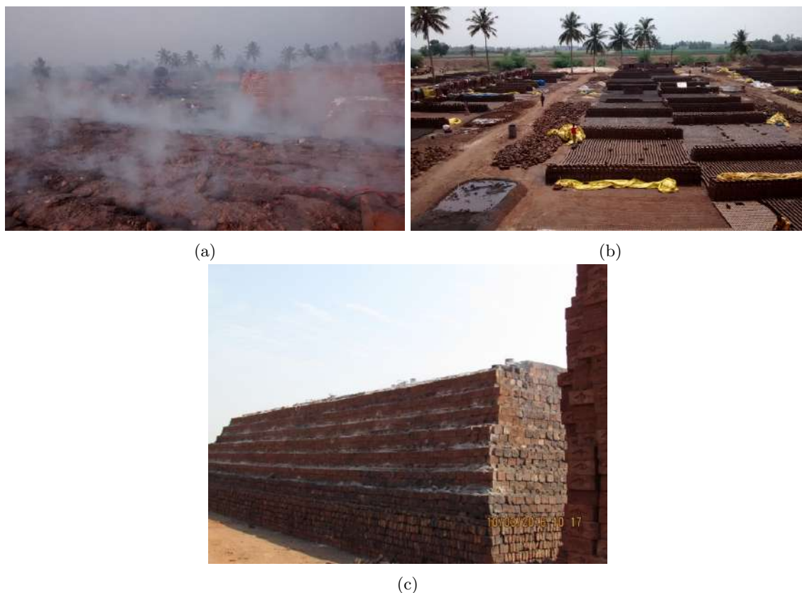
Figure 6: (a) Top view of the clamp measured in Sangli, India. (b) Stacked green bricks for drying. (c) Side view of monitored clamp in Sangli.
